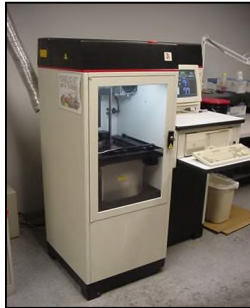
1992 – 3D Systems Stereolithographic printer
